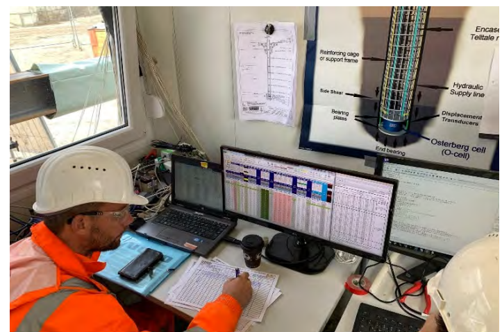
Fugro Loadtest: Static Load test in progress
